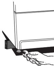
If the dryer is not level, prop up the dryer using a wood block. Use a wrench to adjust the legs up or down and check again for levelness.
